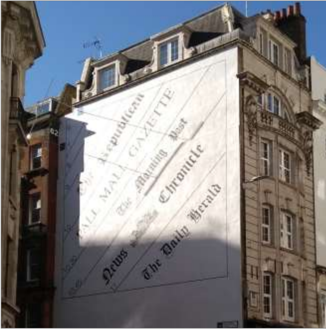
Fig. 6. The finished dial seen from Fleet Street at 11:30 am BST on 21 October, when EoT was 15 minutes, so the dial correctly shows 11:30 + 0:15 - 1:00 = 10:45 sun time.
