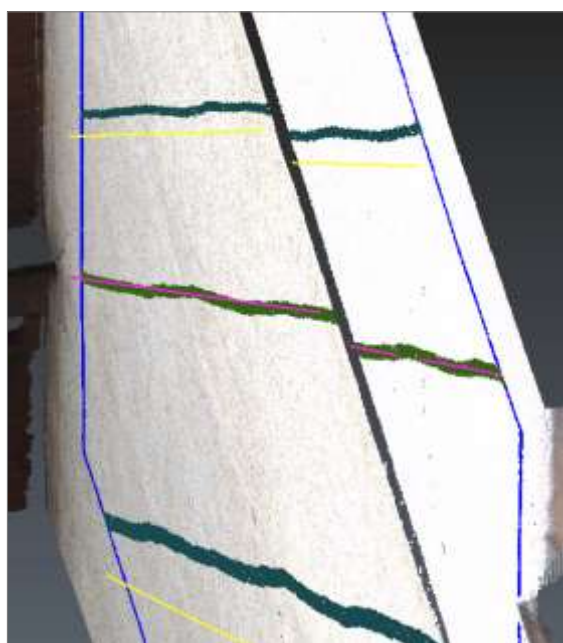
Fig. 3. Oblique view of a true hour 'line' and its best-fit straight line approximation.
